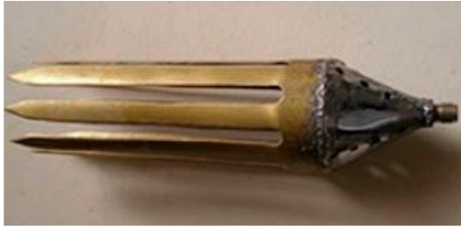
The TDR-150 is an example of a time domain reflectometry soil moisture measurement device.
